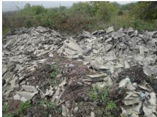
Figures 5 and 6: Asbestos-containing waste placed as a separate pile
