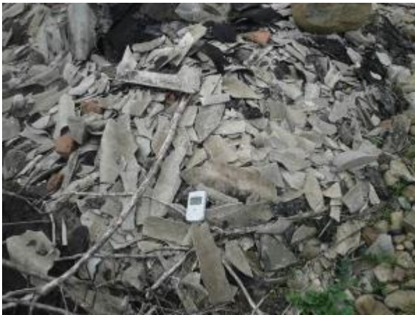
Figures 5 and 6: Asbestos-containing waste placed as a separate pile
